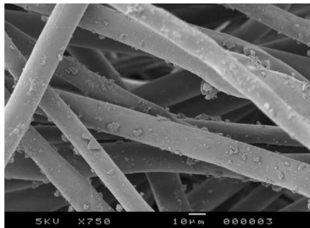
Figure 2. How the filter might appear when viewed with a SEM [5].
